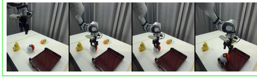
(a) Task: "pick up the poke ball and put it in the tray".  $\pi_0$ -FAST-DROID [L] picks up the distractor (duck) instead (language grounding issue). R1CL- $\pi_0$ -FAST-DROID [R] actually moves the unseen object (pokeball) with only RAG and ICL.
