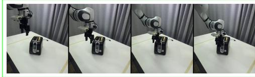
(e) Task: "push the lever on the toaster".  $\pi_0$ -FAST-DROID [L] aimlessly wanders. It cannot figure out the precise location or the grasp (adaptation to a variant of training object issue). R1CL- $\pi_0$ -FAST-DROID [R] completes the precise task, only with RAG+ICL, and with elicited latent actions not in the retrieval data (more information in Section 6). This long-tail task appears infrequently in the DROID dataset.
