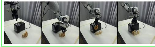
(b) Task: "pick up the bagel and put it in the toaster".  $\pi_0$ -FAST-DROID [L] aimlessly wanders and cannot figure out the grasp or motion (adaptation issue). R1CL- $\pi_0$ -FAST-DROID [R] almost completes the task (only with RAG and ICL) but drops the unseen object (bagel) at the end of the novel motion—a combination of an unfamiliar grasp at its rim, its unique initial vertical position, and the twist-and-lift motion.
